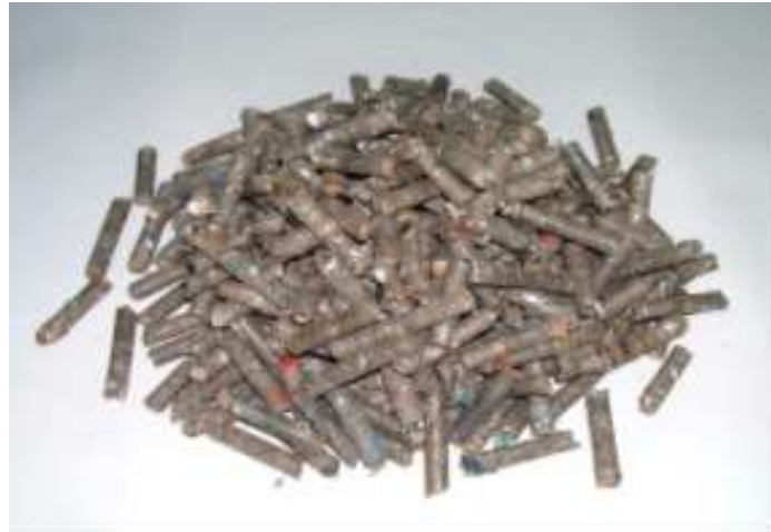
Fig. 13. Solid waste derived fuel manufactured by ITRI (1 cm in diameter, 5 cm long; calorific value of approximately 6,200 kcal / kg)
